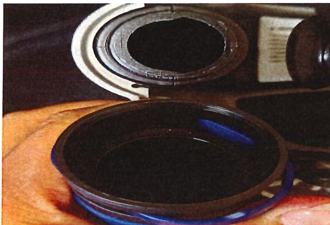
Inspect hood for tears, holes, etc. Insert breathing tube into hood connection. Ensure gasket tube is in place.
